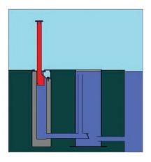
When floodwaters rise, an inlet pipe fills the basin and the flood barrier floats and rises. When the basin is totally filled, an angled support block locks the barrier into watertight position.
