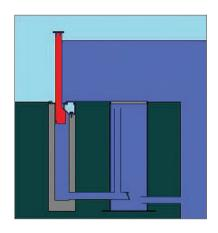
The floodwaters continue to rise without flooding the protected area. When the water subsides, the basin drains using check valves and the barrier returns to its storage position.
